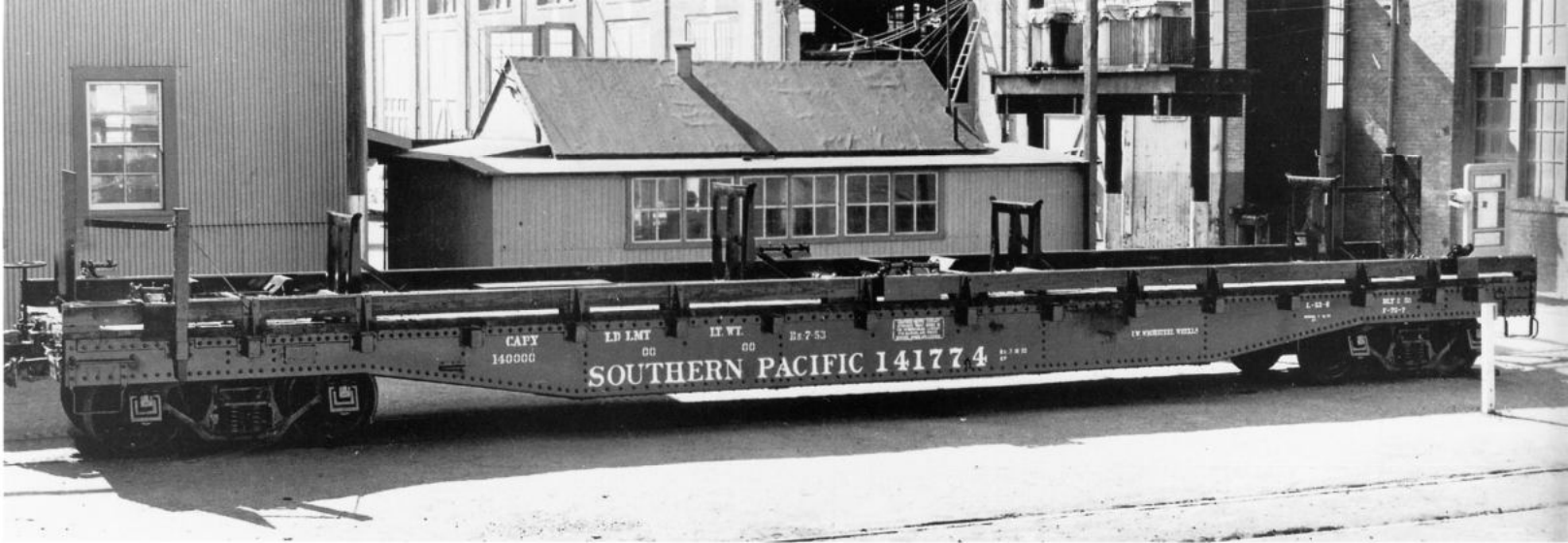
The basic components of early TOFC operations on the Pacific Lines can be seen on this page. Standard 53-foot 6-inch flatcars were used like SP F-70-7 141774 seen, above, shortly after being modified for TOFC service at Bayshore Shops in July 1953. As an extension of Pacific Motor Trucking service, standard P.M.T. 22-foot side-door trailers, as seen left, were used. Loading of the cars was accomplished by means of portable ramps, such as this wooden ramp, seen below at River Team Track in Los Angeles in late 1954. —Above, SP photo, courtesy Tony Thompson; left, SP photo, John R. Signor collection; below, Alden A. Armstrong
