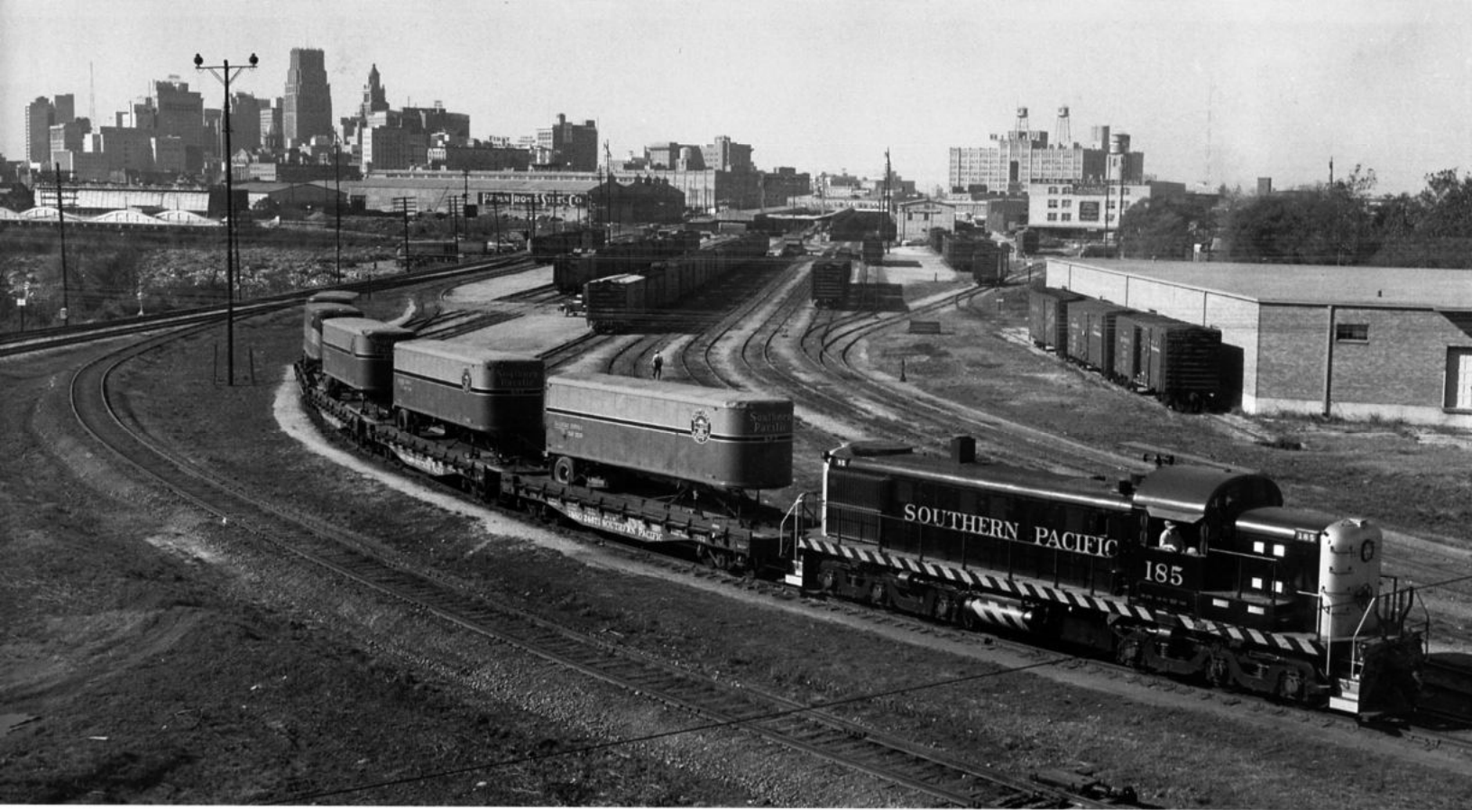
On this page and below opposite are early publicity views of T&NO's piggyback operations in the Houston area during the late spring of 1953. The trailers are a mix of Daylight -painted vans and earlier SPT equipment. Note security bars on the trailers in the lower view. —All, Southern Pacific, John R. Signor collection
