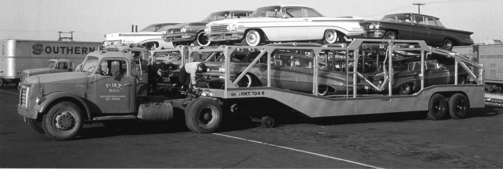
In late 1959, prior to the development of the auto-rack car—or as SP called them, "Auto-Packs"—Southern Pacific began handling finished automobiles in specially-designed PMT auto loaders mounted on Clejan flatcars. In these two views, the first trainload of new 1960 General Motors automobiles has arrived at the West Oakland piggyback terminal on December 16, 1959. SP and General Motors executives were on hand to check the shipments of Pontiacs, Oldsmobiles and Buicks that had been assembled at GM's South Gate plant in Southern California. Once unloaded from the flatcars, it was a simple matter to truck the automobiles to various Bay Area dealers. Compare the difference in design between the PMT trailer above (note Clejan wheel immediately behind tractor wheel) and the more utilitarian designs at left. —SP photos, John R. Signor collection
