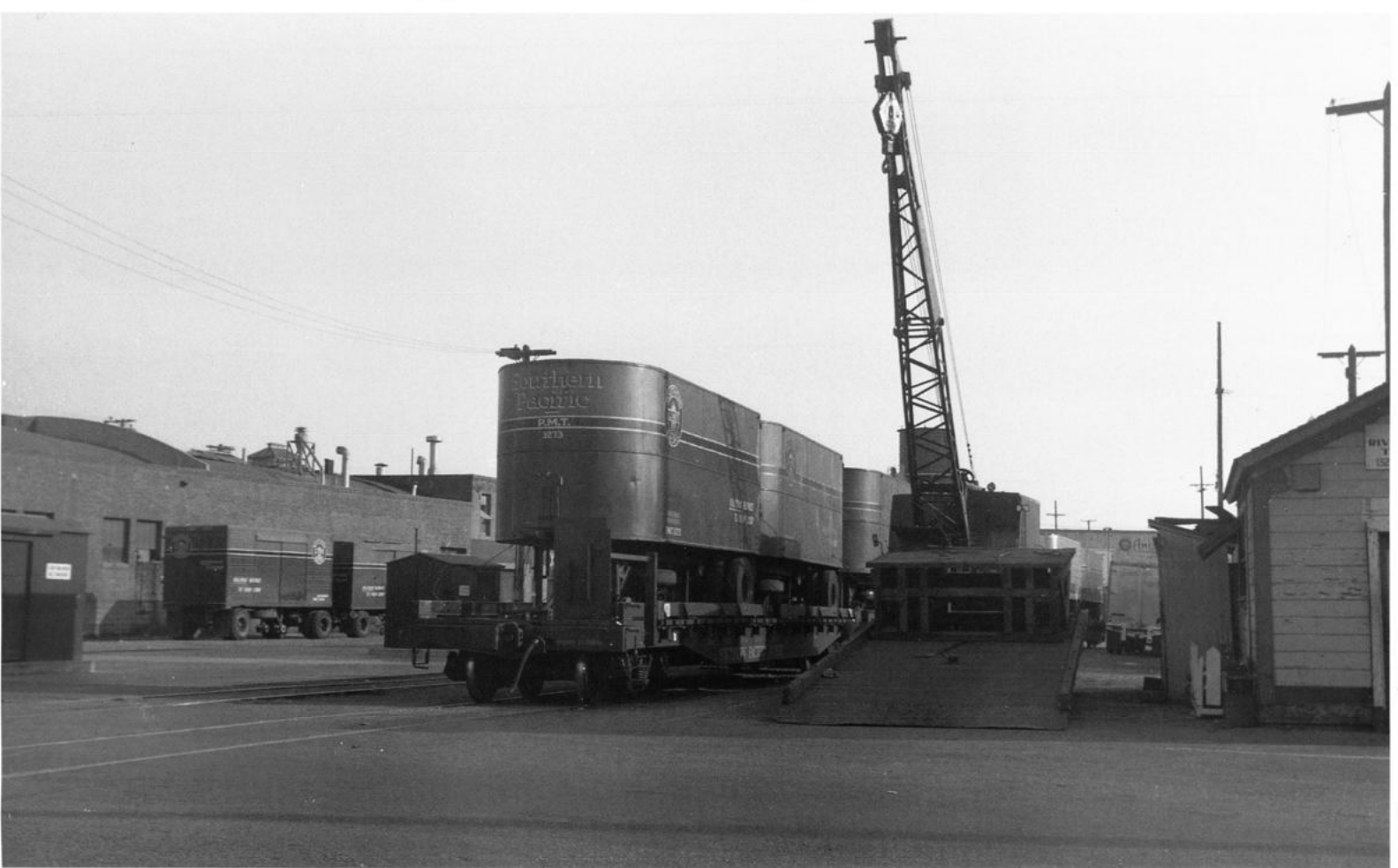
The basic components of early TOFC operations on the Pacific Lines can be seen on this page. Standard 53-foot 6-inch flatcars were used like SP F-70-7 141774 seen, above, shortly after being modified for TOFC service at Bayshore Shops in July 1953. As an extension of Pacific Motor Trucking service, standard P.M.T. 22-foot side-door trailers, as seen left, were used. Loading of the cars was accomplished by means of portable ramps, such as this wooden ramp, seen below at River Team Track in Los Angeles in late 1954. —Above, SP photo, courtesy Tony Thompson; left, SP photo, John R. Signor collection; below, Alden A. Armstrong
