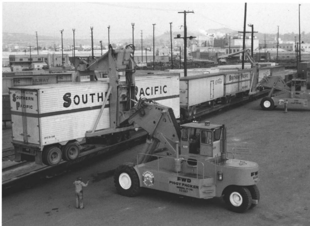
The time consuming operation of loading and unloading flatcars circus style was circumvented by the FWD Piggy Packer. Seen in operation at Los Angeles Shops piggyback yard in October 1966, the Model 70, jointly developed by Southern Pacific Assistant General Superintendent of Transportation Jack Sherbourne, trailer-flatcar crews and FWD, could hoist 70,000 pounds and took normally 5 minutes to unload a car, or 2½ minutes per trailer. —SP photo, John R. Signor collection
