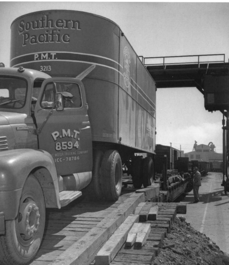
A PMT tractor backs a trailer onto a waiting flatcar at Los Angeles, left, in July 1953. PMT used a trailer hitch system without a kingpin, which required stanchions and cable tie-downs on flatcars. —SP photos, John R. Signor collection
