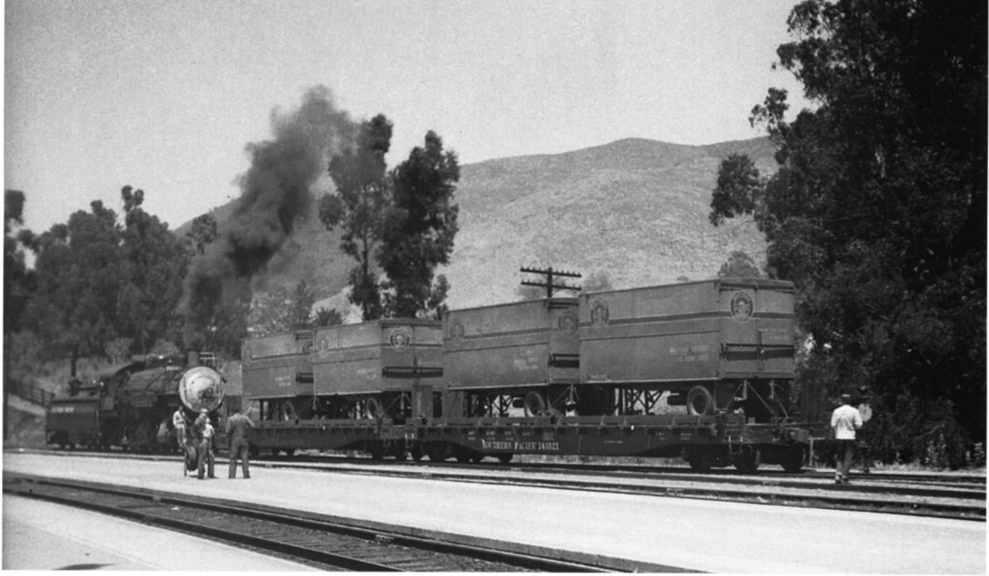
A yard engine prepares to move two recently-modified F-70-7 flatcars loaded with PMT 22-foot trailers at San Luis Obispo in the early summer of 1953. It is speculated that this might have been a test for the suitability of the equipment and tie-down apparatus before the implementation of regular service. —SP photo, John R. Signor collection
