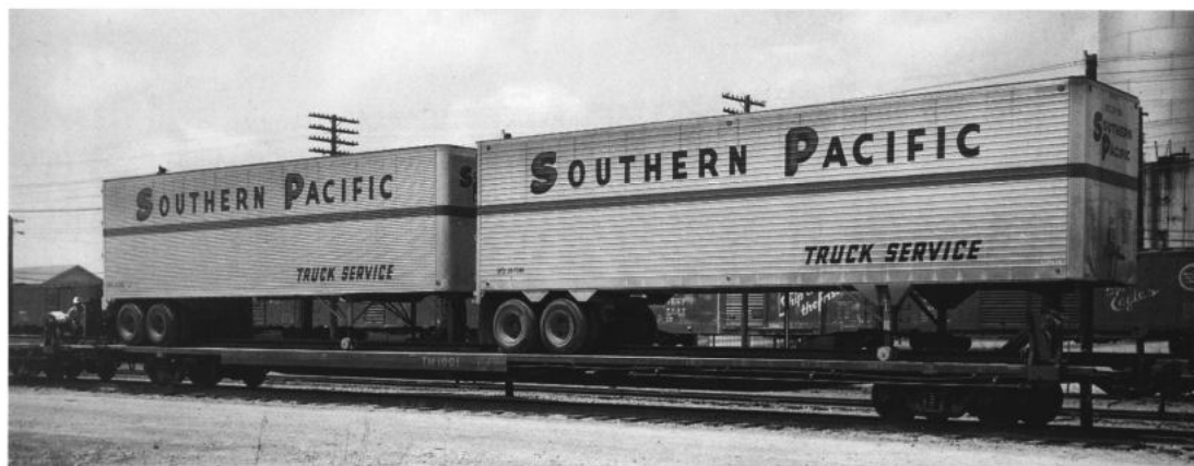
In 1965, as SP operations began to integrate into the national system, a trailing Z was added to PMT/SPT/SWT unit reporting marks and existing piggyback trailers were renumbered to comply with the AAR six-digit number system. Here, a pair of SPTZ trailers, one 35-feet and the other 40-feet 2-inches, are mounted to a Texas-Mexican 85-foot TOFC flatcar, circa 1966. —SP photo, John R. Signor collection
