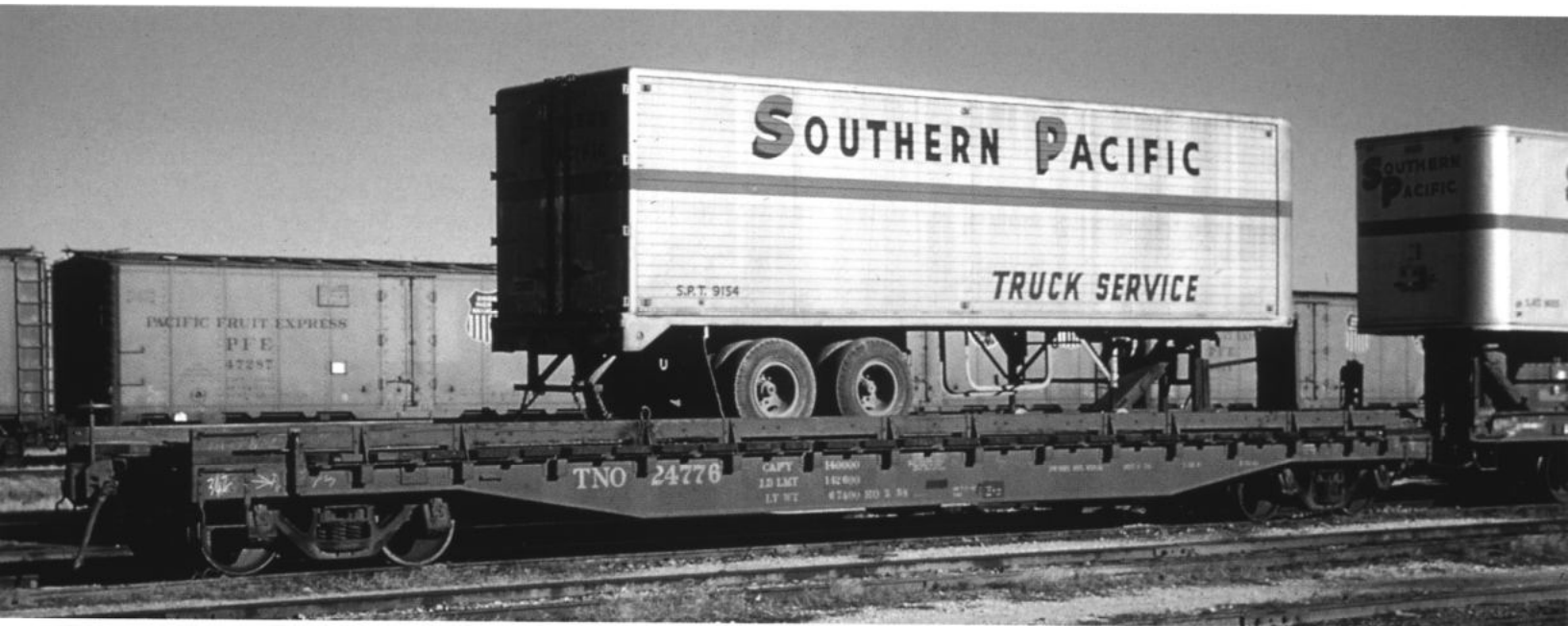
TNO 24776 is seen at Ennis, Texas, on the Dallas Division, January 15, 1961, with a single 32-foot trailer SPT 9154. By the end of 1960, all of the F-70-10 53-foot 6-inch TOFC flat cars had been returned to general service on the Pacific Lines. A few, however, remained in TOFC service on the T&NO for a few more years. — Dick Kuelbs photo, courtesy Rod Loder
