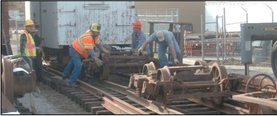
Freight car trucks are shifted to make room for boxcar 706. Photo by Glen Matteson
