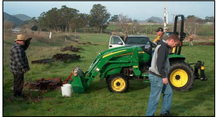
Howard Amborn, Duane Powell and Mark VanKlavern use the improvised forks on Howard's tractor to move track hardware.
