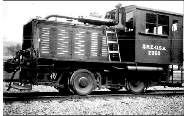
United States Army Quartermaster Corps No. 2050, a twin of No. 2038, was used at Camp San Luis Obispo. This is about as small as you can get and still be a standard-gauge locomotive.
