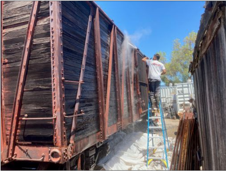
In May, contractor Tom Smith of Advanced Pressure Washing blasts grime from the sheathing boards, in preparation for painting. Brad LaRose photo
