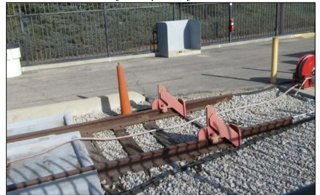
Wheel stop bolted to rail, from San Luis Obispo's roundhouse area, removed with permission of current owner Union Pacific Railroad. Dan Manion photo
